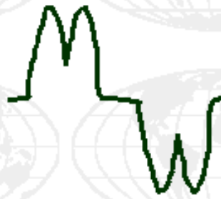
Fig. 4 Actual input current waveform for six pulse VFD with 3% line reactor.
